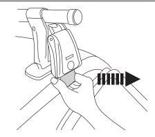
Check clips after installing. Grab each clip and try to pull them hard away from your vehicle, twice. If the clip moves after the second pull, tighten the adjustment post. If the clip still moves after the second pull, recheck your measurements between the towers and adjust if necessary. Check clip again.
