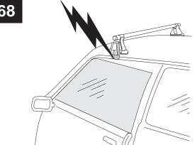
The clip fits tightly between the window and the door frame. Open/close your doors carefully to prevent window contact.
