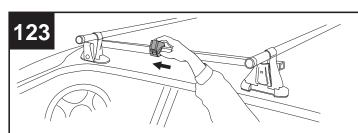
The Stretch Kit must be used with this option. Slide the Stretch Kit housing all the way forward.
