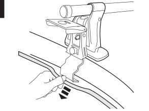
For a secure fit pull down door frame seals enough to insert the clip against underside of raingutter, trim, and/or roof.
