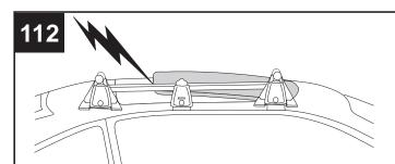
The sunroof should not be opened while the rack is installed. Remove rack when not in use.
