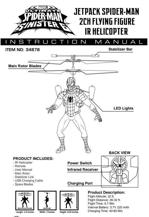
WARNING: Incorrectly storing this RC helicopter may cause the rotor blades to bend and/or warp, which may make it unable to fly properly.
