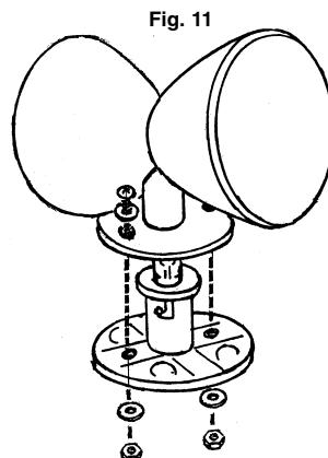
39. Position the new bulb into the socket, depress the bulb and turn clockwise. Make sure the gasket is positioned properly to prevent water and dirt from entering inside the light.
