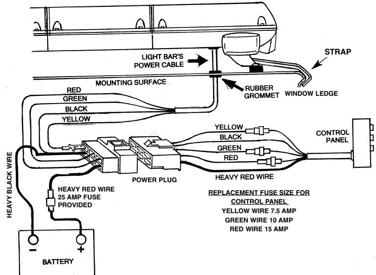
22. Route the heavy gauge RED & BLACK wires to the vehicles battery. If the power wires pass through any drilled holes or firewall, always use a rubber grommet to protect the vehicle.
