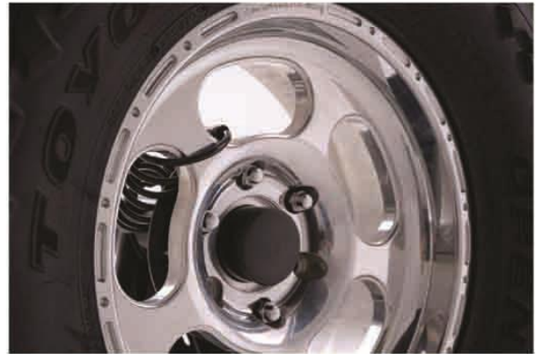
Secure the wheel/tire to the HitchGate using the safety cable through the lanyard safety loop as shown. Figure 4
