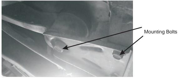
• Once the bushings are removed, check for any burs, fix as necessary
