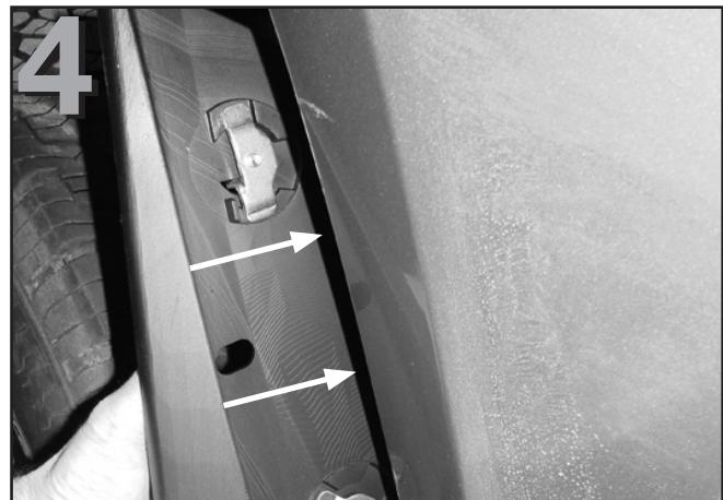
Position the smooth surfaced portion of the MudFlap so that it contours firmly against the fender as shown.
