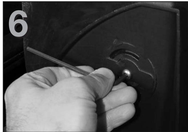
Repeat this process with the top QuickTurn™ fastener.
