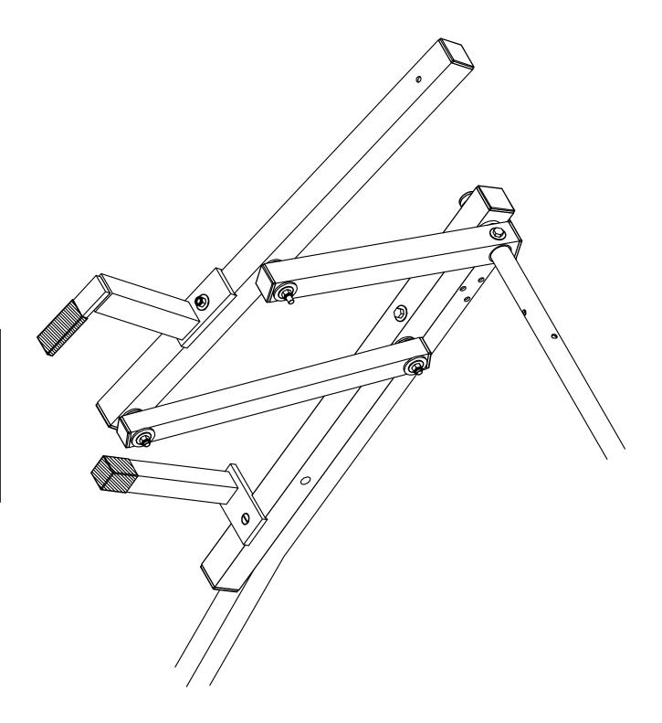
Use the supplied lubricant and coat the pre-assembled Black Plastic Bushing (A). Insert Front Drive Tube (B) into the larger Black Plastic Bushing (C) in the Front Crossmember Assembly (D) so that the black bushings are fully seated.
