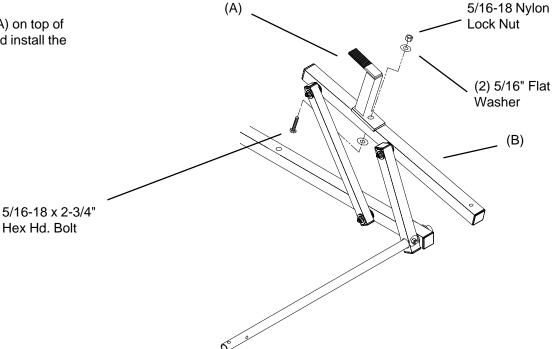
Place the Front Rotation Assembly on top of the Cross-Member (A) and place the Ladder Stop (B) on top of the Lower Rotation Tube, install the 5/16-18 x (4-1/4" or 5") (Flat Hd. Screw). Install 5/16-18 x 4" Hex Hd. Bolt through Lower Rotation Tube and through the Cross-Member.
