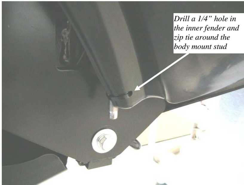
Figure 19 Left side inner fender tucked into bumper
