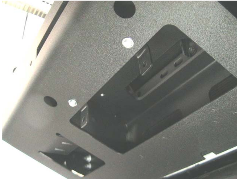
Figure 21 License Plate Brackets installed
