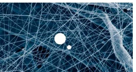
Conventional cellulose fibers are larger than PowerCore® Ultra-Web® nanofibers, and have larger spaces between the fibers, causing contaminant to load in the depth of the media plugging the airflow path; resulting in higher restriction and less capacity.
