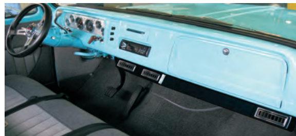
1964-66 Chevy dash shown with rotary controls
