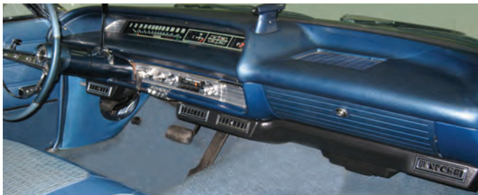
1963 Impala dash with SureFit kit (note: SureFit installations in factory air equipped Impalas use the original in-dash A/C louvers.)
