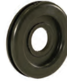
33133-VUI Rubber grommet inner hole size .500", 1.5" O.D. - drill hole size 1.25"
