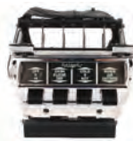
OEM '57 Chevy deluxe control with the supplied Electronic Cable Converters™ installed from our Gen IV kit.
