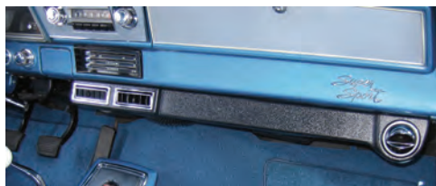
1966-67 Nova dash using factory controls
