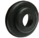
33137-VUI Rubber grommet inner hole size .625" (will expand to 1"), 1.75" O.D. - drill hole size 1.25"
