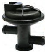
46103-VUH 3 Vacuum heater control valve (normally closed - vacuum to open)
