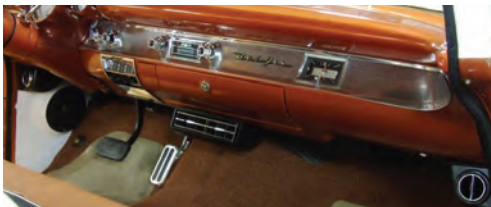
1957 Chevy installation with center plenum.
