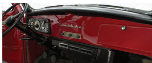
Studebaker C-Cab dash with Climatizer System
