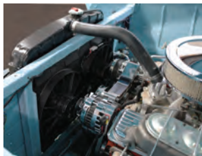
371255 3 -Tri-Five Chevy Dual Cool™ fan package designed for 6 cyl. radiator position as shown.
