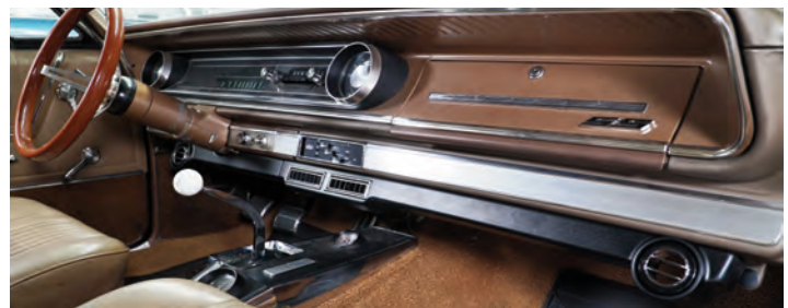
1966 Impala dash with included under-dash louver pods
