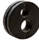
33134-VUI Double-hole rubber grommet for #6 & #8 hardlines. 1.562" O.D. - drill hole size 1.25"
