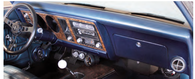
1969 Firebird-factory air dash with SureFit kit
