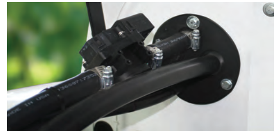
Vintage Air SureFit system evaporators install completely inside the cab for a clean, original looking engine compartment. Firewall plate mounts to original holes.
