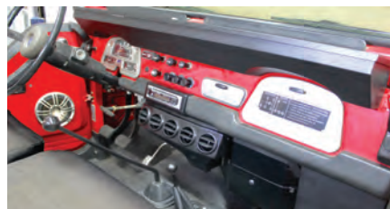
U.S. spec Toyota FJ-40 Land Cruiser dash using factory controls and Vintage Air louvers.
