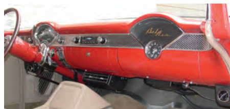
1955-56 Chevy installation with center plenum.
