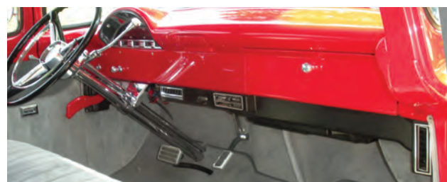
Under dash panel with louver package shown is available with or without control panel installed.
