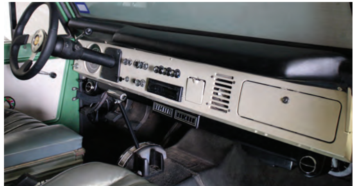
Ford Bronco dash with SureFit system with full width plenum, controls and Vintage Air louvers. 4-vent kit also available.
