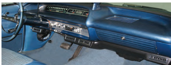
1963 Impala dash with SureFit kit. (Note: SureFit installations in factory air equipped Impalas use the original in-dash A/C louvers.)
