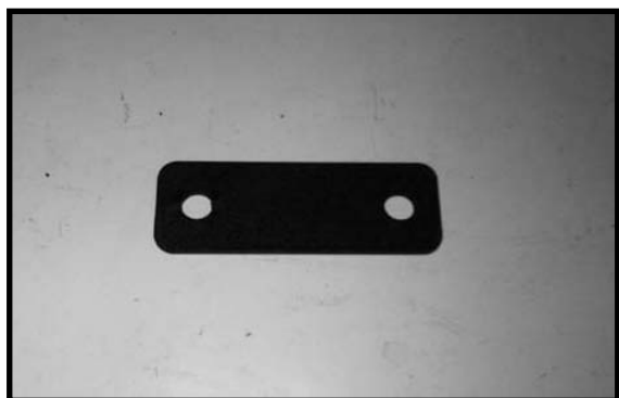
56070-18 / Qty (2) Emergency Brake Cable Bracket
