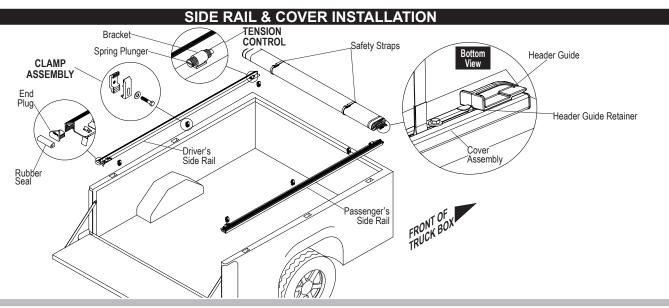
STEP 1: Attach the TruXedo rails to the truck's vertical inside flange as shown in Detail A. To get the correct TruXedo rail alignment from front to back, See Detail-B. Compress the rear D-seal against the closed tailgate and hold. Attach clamps starting at the tailgate. Evenly space 3 clamps along each TruXedo rail, leaving approximately 8" on each end.
