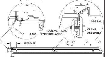
For optimum latching performance and cover fit, side rails must be level. To adjust rails, loosen screws and reposition male clamps higher or lower. Tighten all clamps.
