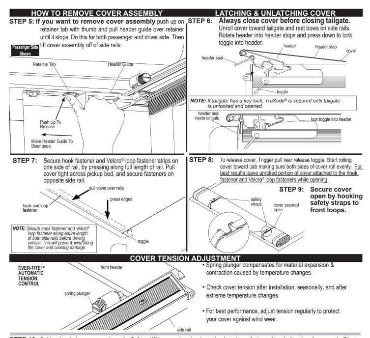
**STEP 10:** Set tension during **warmest part of day.** With cover closed, release hook and loop fastener from both side rails near cab. Check compression of both spring plungers against the front header per diagram. Roll cover open and make adjustments. Close cover and re-check adjustment. Repeat until satisfactory tension has been achieved.
