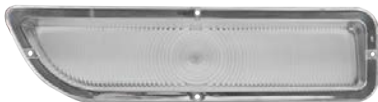
A9834 '62-'66 GMC Parking Light Lens Clear, (Has original chrome look around outside edge.)
