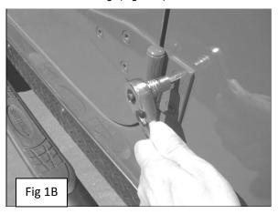
3. When you remove the lower door hinge a backing plate (figure 2) will come loose. Enter the Jeep from the opposite side to access the plate. You will need it in step 4.
