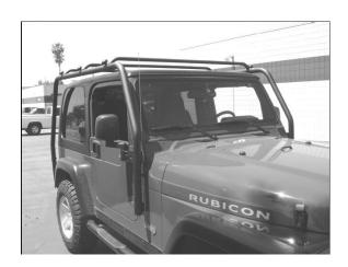
17. Installation is now complete. Note: After driving the vehicle with the rack a few days it is recommended to check all of the bolts for proper tightness. If loose, retighten.
