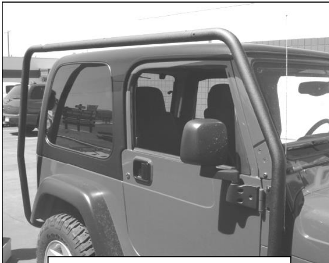
Figure 6 – Uprights installed but not tightened – Important, do not tighten until the cross bars are installed.
