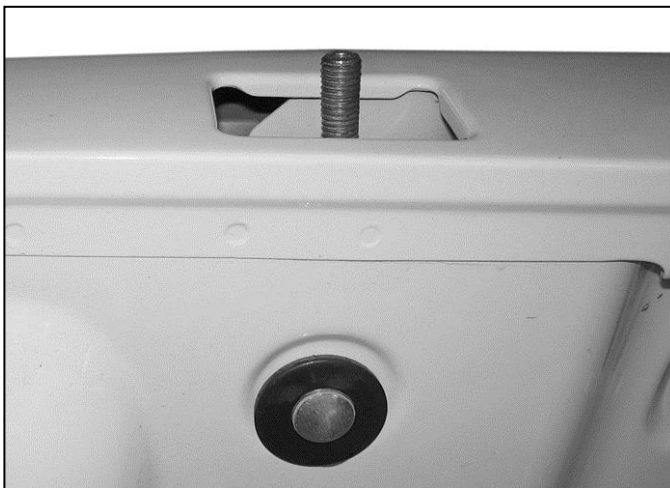
(Fig 4) Use the "J" Bolt to secure the front mounting holes on the Bracket to the stake pocket if possible. Do not drill any mounting holes until after all mounting locations are checked for clearance
