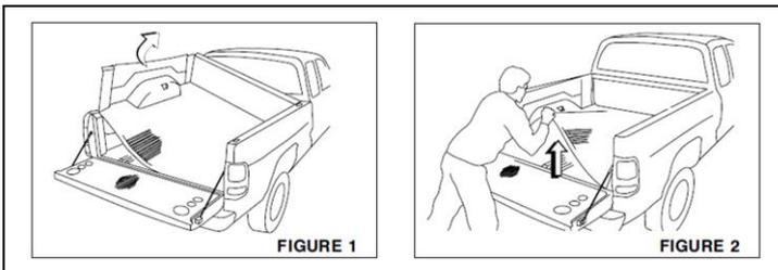
**(NOTE: Some bedliners may not have front rail lip. These require two (2) screws to secure front wall.)**
