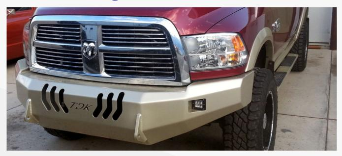
For Dodge or Ram 1500 - 3500 models dating back to 1994 and 1500 - 5500 models dating back to 2006, Throttle Down Kustoms has a custom bumper option available. All TDK bumpers are CNC laser cut, MIG hand welded, and built with solid PNO steel plate to ensure the highest quality possible. They're built to withstand hardship, strain, and exposure to the harshest conditions, and they all come with a lifetime warranty. Plus, as always, they are customizable.
