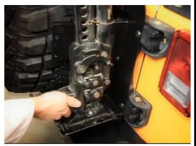
Insert and hold the supplied aluminum spacer between the lowest hole on the jack handle and the threaded bung in the Accessory Mount. Thread the supplied 3/8" x 2" bolt with washer through the jack handle and spacer, and into the threaded bung. Do not tighten yet.
