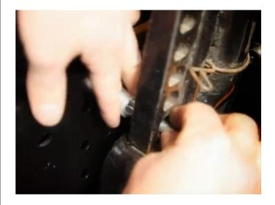
Insert the supplied 3/8" bolt with washer through the bottom side of the slot in the Accessory Mount pedestal and upward through the rear-most hole in the foot of the jack. Thread the supplied 3/8 serrated nut with lock washer onto the bolt.
