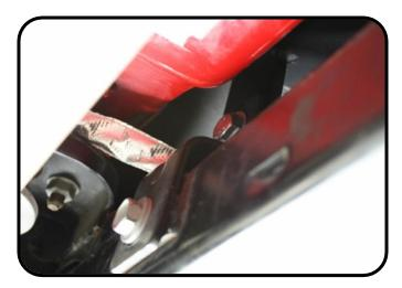
Note: There is some "play" in the bumper after all the bolts are installed and finger tight. This is to allow room for slight variations in mounting points from Jeep to Jeep. Visually inspect the bumper and adjust and align if needed.
