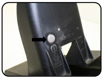
5. Use the factory screws to position the extension bracket as pictured. Use the holes closest to the middle of the extension bracket.
