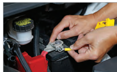
NOTE: Some vehicles may require grounding and/or direct connection to the battery.
