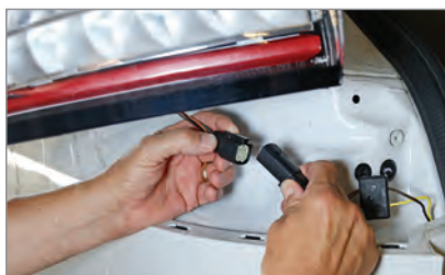
4. Plug the tail light into the T-One® connector.
