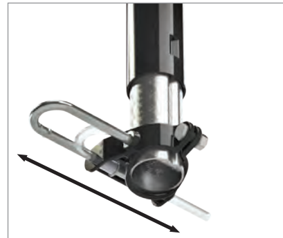
Spring loaded drop leg pull pin
