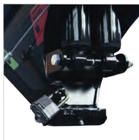
Lockable BULLDOG® coupler for added security
