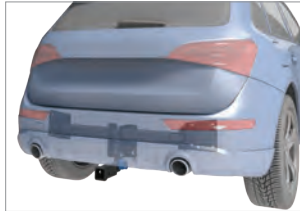
Euro Hitch installed with receiver box inserted
