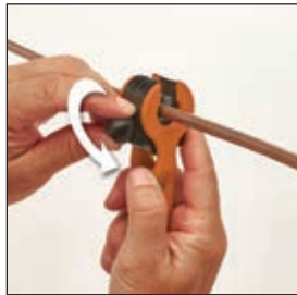
Spring-loaded automatic cutter: touch blade to tubing, turn dial 8 times, cut tubing
