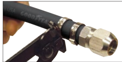
Thin head for crimping in tight spaces
