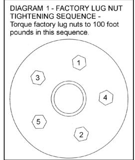
**WARNING:** When the tires / wheels are installed, always check for and remove any corrosion, dirt, or foreign material on the wheel mounting surface, or anything that contacts the wheel mounting surface (hub, rotor, etc.). Installing wheels without the proper metal-to-metal contact at the wheel mounting surfaces can cause the lug nuts to loosen and the wheel to come off while the vehicle is in motion.
