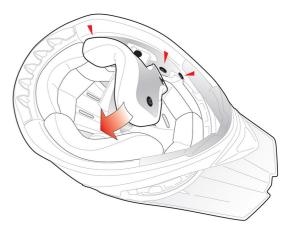
The cheek pads are easily removable also in case of accident through a red strap which removes the cheek pad even if the helmet is worn by the rider.
