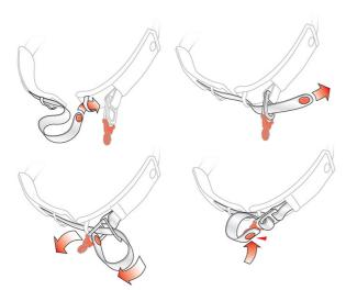
The **D-RING RETENTION SYSTEM** has been designed and patented by Suomy. Insert the free side of the strap in the rings. Pull the end until the strap presses firmly against the jaw.
