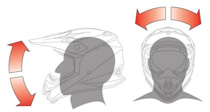
To have a maximum safety the <u>helmet</u> must fit tightly and be correctly and securely fastened, in order not to be able to be taken off neither by pulling it nor by rotating it around the head.
