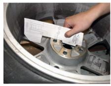
5. Lay the template inside the wheel as shown.
