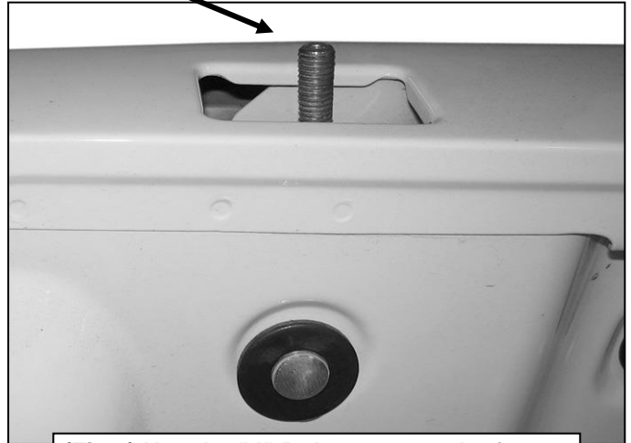
(Fig 8) Use the "J" Bolt to secure the front mounting holes on the Bracket to the stake pocket if possible. Do not drill any mounting holes until after all mounting locations are checked for clearance
