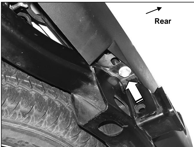
(Fig 1) Factory bumper may be attached to top of tow hitch. Remove factory hex bolts as required.
