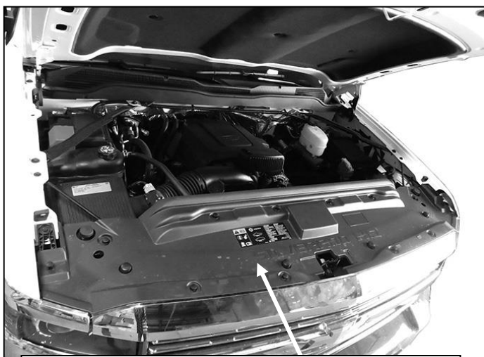
(Fig 9) Remove plastic cover on top of grille
