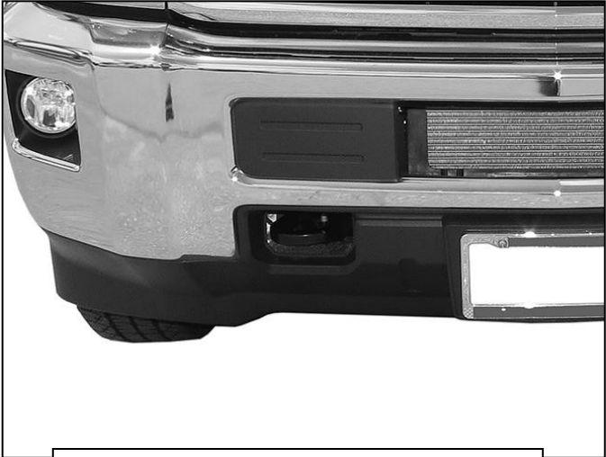
(Fig 1) Opening for tow hook pictured
