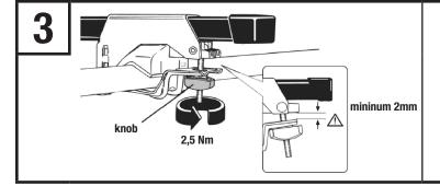
Tighten the knobs firmly (torque 2,5 Nm), and check that the gap is at least 2 mm in each case. If the gap is less than 2 mm, unscrew the knobs and hook the brackets into a higher set of holes.
