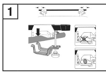
Position the load bars on the roof rails with a minimum spacing of 700mm.
