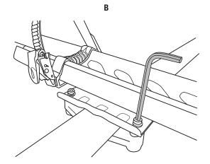
Slide rear mounting under bracket under the load bar (square, oval or round) and attach to the rear mounting plate with bolts and washers like in prior step.
