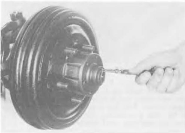
Figure 7 Remove snap ring and drive flange screws.
