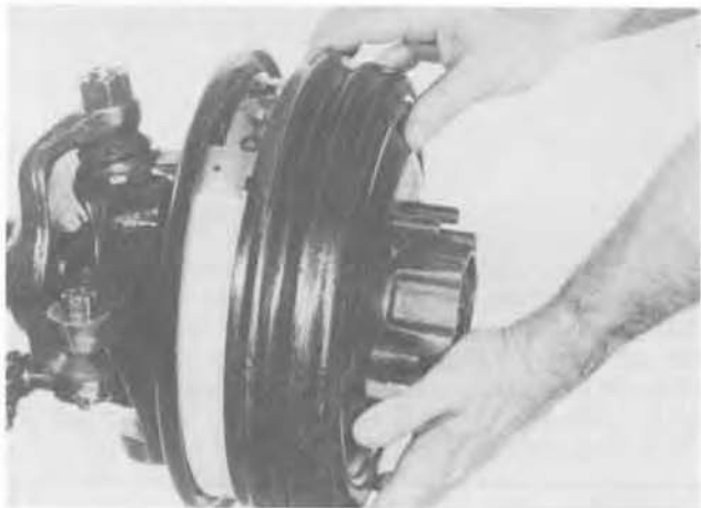
Figure 10 Remove drum assembly. Outer wheel bearing will slide out as drum is removed.
