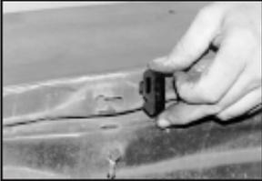
Hood bumpers are a must for proper hood fit. Note slot in fender and matching anchor on rubber bumper. Just slide the bumper anchors through “key hole” into slot, and you’re finished.
