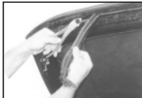
4) Once all the weatherstripping is removed you must carefully clean the metal surfaces of the top irons so the new adhesive will hold firmly.
