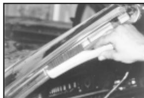
4) A wire brush can be helpful in removing small or stubborn particles. Watch out for sharp edges, and be careful not to scratch your channel.
