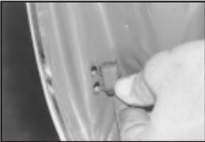
To install door bumpers, align arrowhead-type anchors with holes in door and push in with thumb. It may be necessary to insert a blunt object in the bumper hole to put pressure on the anchor heads to pop them through the holes. Be careful not to tear the rubber. Water or Windex will help lubricate the part.
