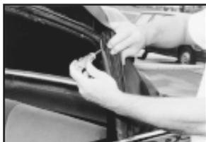
3) Next, remove the header seal (the seal against the windshield top). It is fastened with nylon pins that will tear out and have to be removed with side cutters (some models also use glue). Your new part has them installed.
