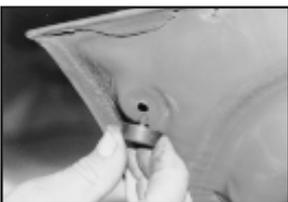
Replace flattened, cracked and hardened trunk bumpers by popping out the old ones with a screwdriver. Line up the anchor tip with factory hole, and push. With a little water or Windex for lubricant, thumb pressure is all you will need to install new trunk bumpers.
