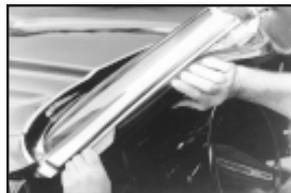
8) Once the strip is fully inserted, install the screws or black plastic anchor pins at the other end. Repeat the same steps for the other side of the car, and you're finished.
