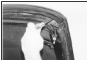
1) Begin by raising the top to a comfortable working position. Remove the screws at each front corner that anchor the weatherstripping to the top irons.
