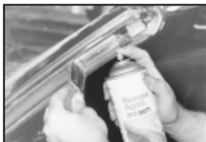
2) Now remove the three sections of weatherstripping on each side rail of your top. They are held in place by screws and factory adhesive. Remove the screws and pull off by hand. Use 3M Release Agent if necessary. You may find it necessary to raise or lower the top to gain access to the screws in the rear piece.
