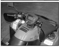
NOTE: If machine has *handle bar warmers, remove existing fastener* in end of grip and reuse it to attach **H**AND **C**UFFS<sup>™</sup> to handle bar (plastic fasteners will not be used).
