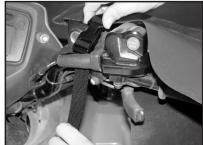
4) Insert plastic fastener in grommet on Hand Cuff and align point in center of rubber grip. With Phillips screw driver, thread fastener into rubber grip until snug. See note at bottom if machine has handle bar warmers.
