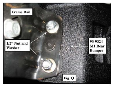
achieved, torque the 1/2" bumper mounting hardware to 85 ft./lbs and the **OE** hardware to manufacturers specifications. (Fig Q)
