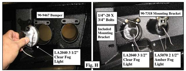
Step 16: Install the fog lights into the new M1 front bumper (93-9467) using the supplied (4 per side) 1/4"-20 X 3/4" bolt and hardware. (Fig H)
