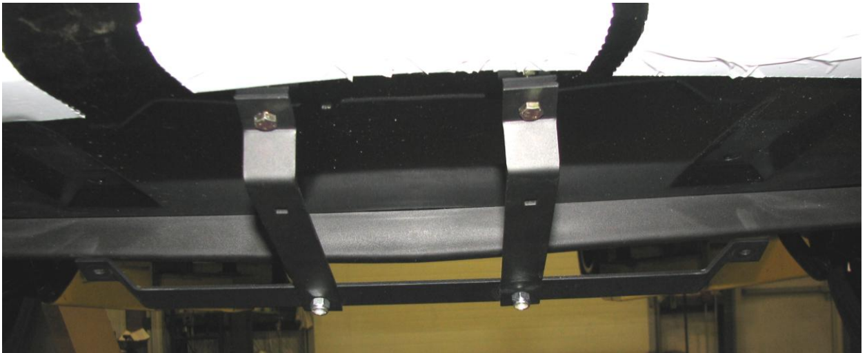
Figure 3: Insert the M6 bolts into the fascia and tighten flanged Nyloc nuts
