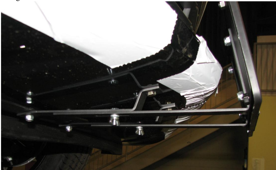
Figure 5: Installation of license plate assembly to vehicle
