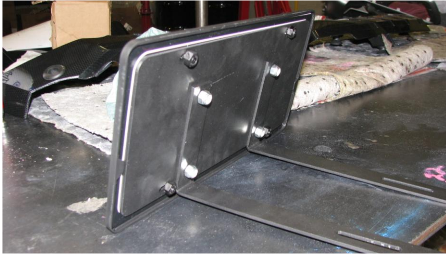
Figure 4: Assembled license plate, plate mount, and plate mounting arms
