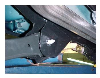
**Step 3:** Take the T-shaped nut plate and slide it into the driver's side motor mount through the top opening. Once the nuts can be seen through the two holes in the lower side of the motor mount, the tab may be folded over to hold the nuts in position. It is helpful to give the tab a slight arch before inserting it into the motor mount.
