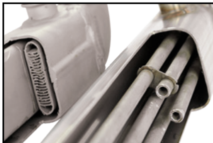
Stock Factory EGR Cooler with mesh vs. Sinister EGR Cooler with proprietary tube design
