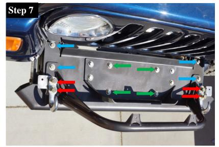
Working from the base of the front bumper install your options on top of each other as follows: Winch Guard >> Light Tabs >> Recovery Hooks at the very top. Any option you may not have can be eliminated from the installation.
