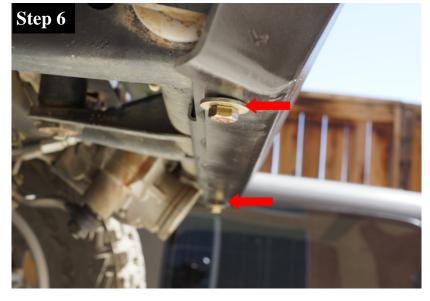
Slip the front bumper onto the frame horns and loosely install the (2) 1/2" - 13 x 1-1/4" HHCS and (2) 1/2" Washers as shown in the red arrows. Do not tighten at this time!
