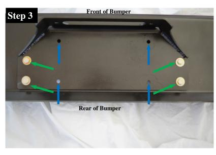
With an aftermarket swaybar installed we recommend installing your fairlead mount in the rear position as shown.
