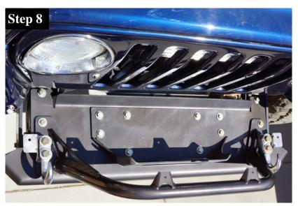
You are now ready to fully tighten your front bumper. Torque the following bolts as shown:
