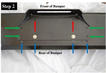
The OEM swaybar will be installed on top of the bumper with the swaybar running across the rear mounting holes identified by the blue arrows.
