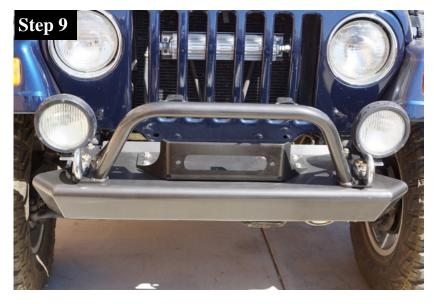
Complete you installation by reinstalling your factory fog lights on optional Light Tabs or on the Winch Guard.
