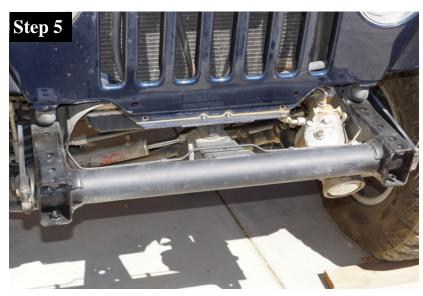
To install the Savvy Front Bumper you must remove your fog lights, tow hooks, OEM swaybar cover, OEM swaybar (if applicable) and current front bumper.
