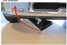
8. Slide the Scoop Assembly up into the bottom of the air box at angle that allows the support tab to slide into the scoop channel.
