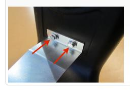
5. From under the truck; remove the bumper mounting nut using a 18mm socket.
