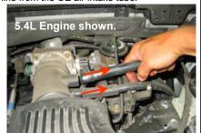
8. Unclamp and open the air cleaner to gain access to the MAF housing.
