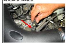
**21.(a)** On **4.6L Engines:** Cut the 3/4"x6" hose down to about 3" to bridge the upper port on the intake tube to the air bypass valve, secure with #8 hose clamps.
