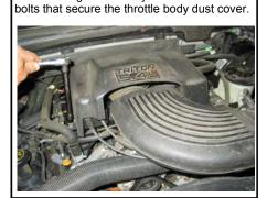
5. At the throttle body, loosen the hose clamp on the OE air tube.
