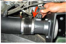
**23.** Install the S&B air filter and tighten hose clamp.
