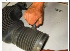
**14.** Install the rubber grommet provided into the S&B intake tube and then carefully insert the air temperature sensor into the grommet
