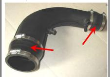
**19.** Install the S&B intake tube onto the throttle body and MAF sensor housing.
