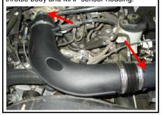
**20.** Reconnect the air temperature sensor electrical connection..
