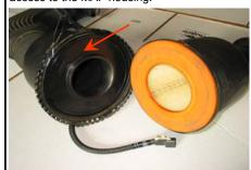
Assemble the MAF sensor, heat shield and the filter adapter using the two gaskets and 1/4-20 x 1" bolts provided.
