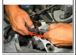
10. Release the four clips that secure the MAF sensor housing by pushing with a flat blade screwdriver. Remove the housing and set the wiring harness aside for now.
