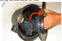
Disconnect the electrical connection for the air temperature sensor.
