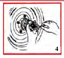
Re-install cover assembly with its gasket. Tighten cover screws or hex bolts to 3.0-4.0 N~m (26-35 in. lbs) using torx wrench "T15".
