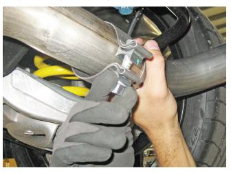
5. Place the band clamp (10-0338) over the exhaust tip and slide the tip over the muffler. Torque the band clamp to 30 Nm once the tip is in position.
