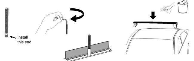
3. Install the Gasket Pads onto the cross bar-FPE end supports at the indicated positions. Install the cross bars onto the vehicle as directed in the FPE end support instructions.
