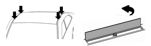
2. Install the fixed point set screws. Tighten to 2Nm (hand tight). Apply the spacer tube over the set screw (if required). Clean and dry the roof area where installing.
