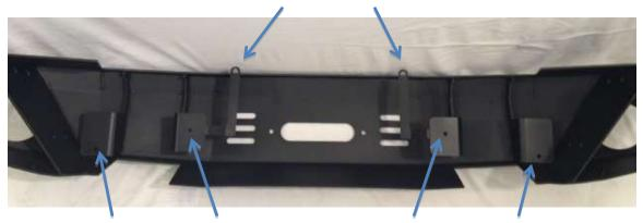
Use a 9/16" wrench/socket to secure <u>4</u> 3/8" bolts, <u>8</u> 3/8" washers, <u>4</u> large washers, <u>4</u> 3/8" nuts
