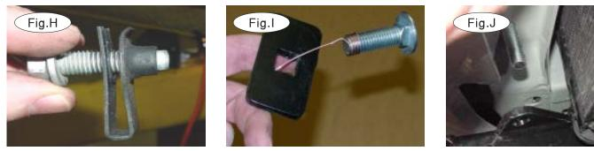
5. Remove the spring nut clips from the bottom of the bumper core (Fig.H).
