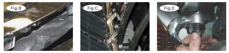
2. Important: please use all supplied bolts and parts and read all instructions carefully before beginning this installation. The majority of questions you may have can be answered within the text, and proper installation will ensure safe and secure travel. Now, begin the installation by snapping loose the top of the chrome grille (Fig.B), then pulling forward then up and out (Fig.C). This will allow easy access for the steps that follow.
