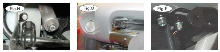
10. Remove four 18mm (head) bolts holding the sway bar to the frame on each side (Fig.N,Q), then let the stabilizer bar fall out of the way.
