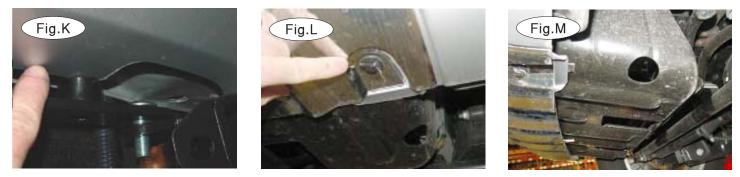
7. Put  $\frac{1}{2}$ " x  $1\frac{1}{2}$ " carriage bolts in the ends of the center brace then bolt the center brace into position with  $\frac{1}{2}$ " nuts and lock washers using two  $\frac{1}{2}$ " spacers between the bumper core and the center brace (Fig.K). Trim the fascia corner slightly near each spacer for clearance.
