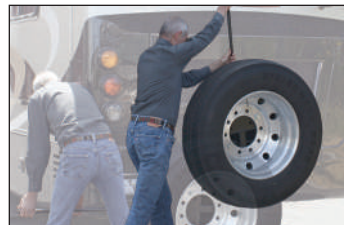
A patented hinge mechanism makes raising or lowering the spare easy.
